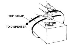
2. While standing to one side of the strap line, hold the hand tensioned strap in position with your left hand, grasp the tool in your right hand and squeeze the handle to the base, thus, lifting the feedwheel. Position the rear foot over the strap and then slide the front foot under the overlapping ends approximately 1" ahead of the lower strap end.
