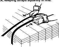
While standing to one side of the strap line, hold the hand tensioned strap in position with your left hand, grasp the tool in your right hand and squeeze the handle to the base, thus, lifting the feedwheel. Position the rear foot over the strap and then slide the front foot under the overlapping ends approximately 2"-4" ahead of the lower strap end.
