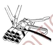
6. Break off the strap at the seal by raising the tool perpendicular to the seal, then lowering it.
