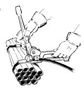
5. Notch the seal with a Delta sealer to complete the joint.
