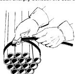
Squeeze the handles together to lift the feedwheel. Insert the strap into the slot of the breaker nose and push the tool up against the seal.
