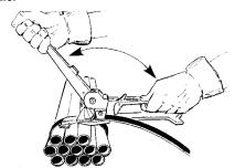
4. When desired tension is reached, push the drive pawl forward and rotate the tension handle back to contact the lift arm.
